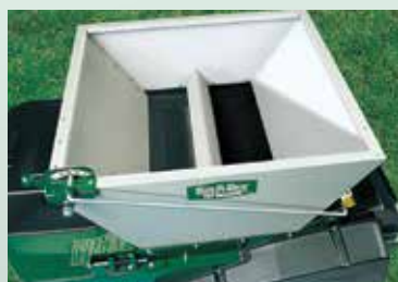
Galvanized hopper means no rusting—or potential rust flakes in topdress material.
