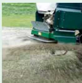
WideSpin technology with 0-15° adjustable spinner angles broadcast from 20 ft to 40 ft.
