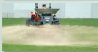
Adjustable spinner angles— up to 26° up or down.
