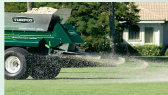
Adjustable spinner angled down for better turf penetration.
