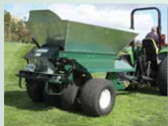
Four-wheel walking beam suspension.
