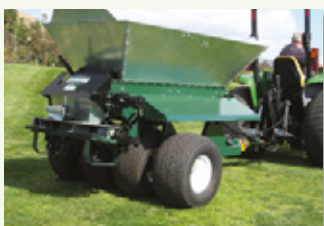
Four-wheel walking beam suspension.
