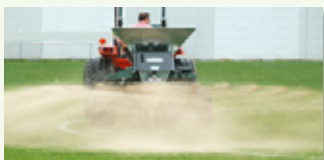
Adjustable spinner angles—up to 26° up or down.
